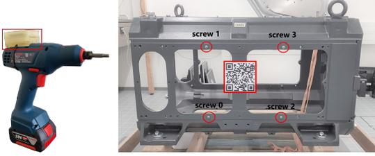
Figure 2: Electric screwdriver with attached sensor module (red circle) and motor-block with four screws (red circle) and encoded marker (red rectangle).
