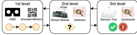
Figure 4: Our quality metric detection in three stages: Process level *coarse-grained monitoring*, *fine-grained monitoring* of the task, and *fine-grained monitoring* of each action.
