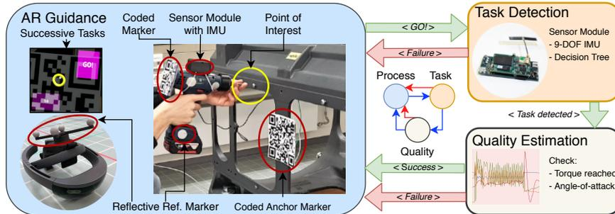
Figure 1: Users wear HMDs and use a sensor-augmented hand-held tool. They follow the task-by-task guidance to complete manufacturing processes. We continuously monitor the process, detect and classify actions, and extract quality metrics via ML.
