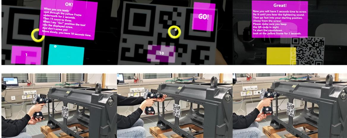
Figure 5: Visualization of one step from a larger process: First, the user is instructed on the next step. Then when ready, the user positions the tool within a given time frame, and finally performs the task. We use the direction of gaze and countdowns for progressing through the process guidance system.
