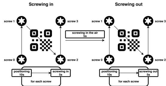
Figure 3: Worker guidance example with sequential work steps, e.g., positioning a tool and executing of tasks such as tightening screws. *Screwing in the air* is executed position-independent.
