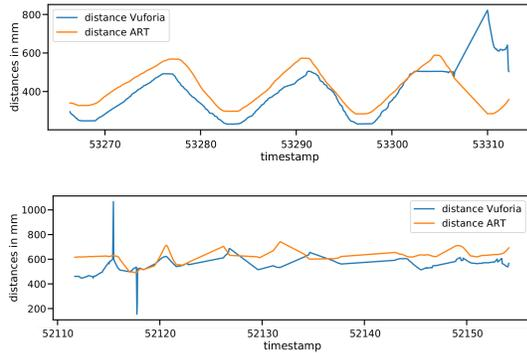
Figure 6: Top: Tool moves back to front in a range of 80cm. Bottom: Random slow movement of tool with SLAM enabled.
